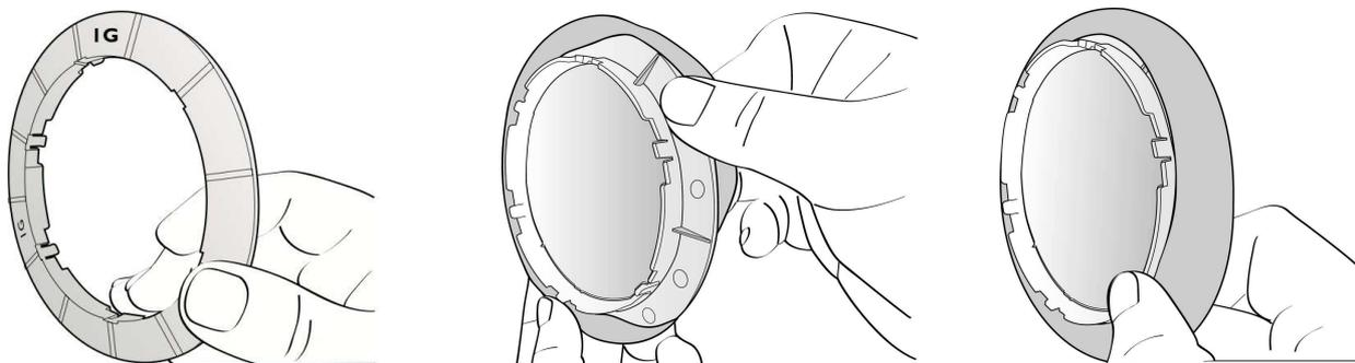
2. Put cleaning ring onto cleaning wheel correctly (luck 6 claws) for no leakage.
